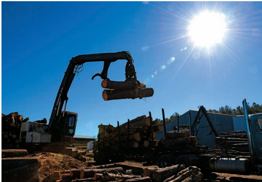
The knuckle-boom loader unloads pine logs at S & S Farms
